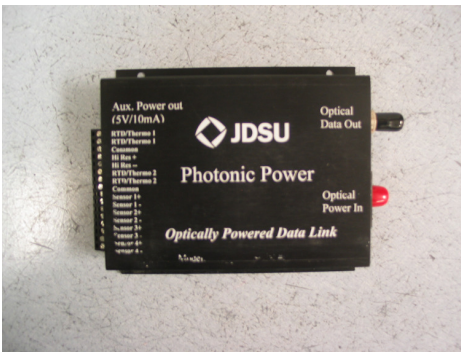
Optically-powered remote module processes up to 7 metering, protection and temperature channels simultaneously
