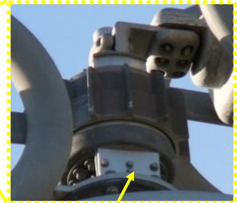
Optically-powered Remote Module powers the measurement electronics
