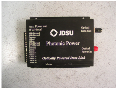
Optically-powered remote module with up to 7 simultaneous channels
